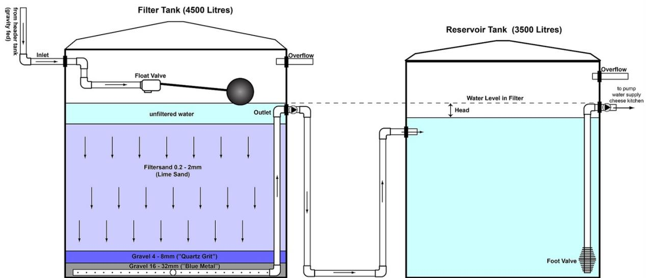
Figure 1: Schematic drawing of the Water Filtration System (see text for explanations)
