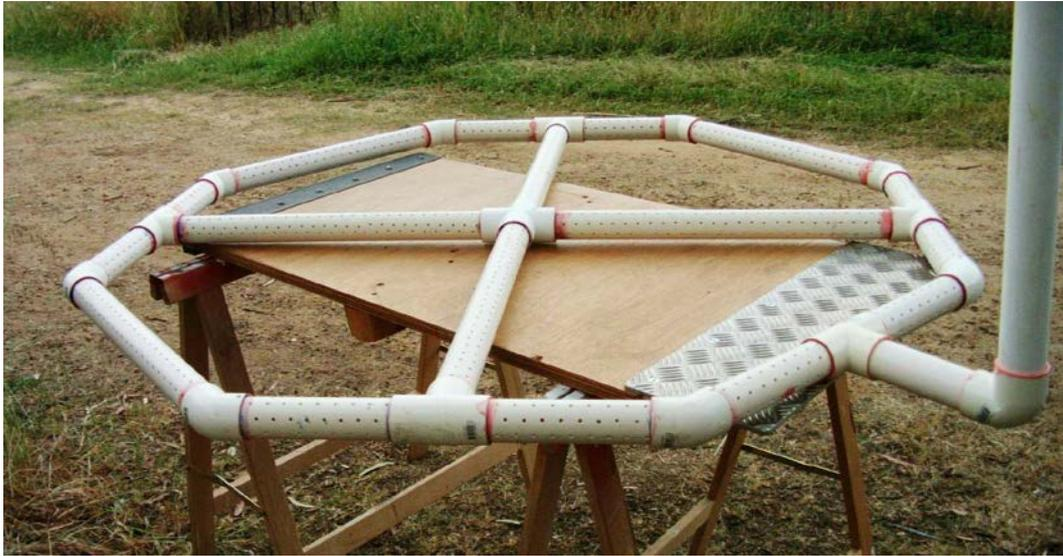
Figure 3: Assembly of perforated 40mm PVC pipes and joiners, which collects the filtered water at the bottom of the filter tank
