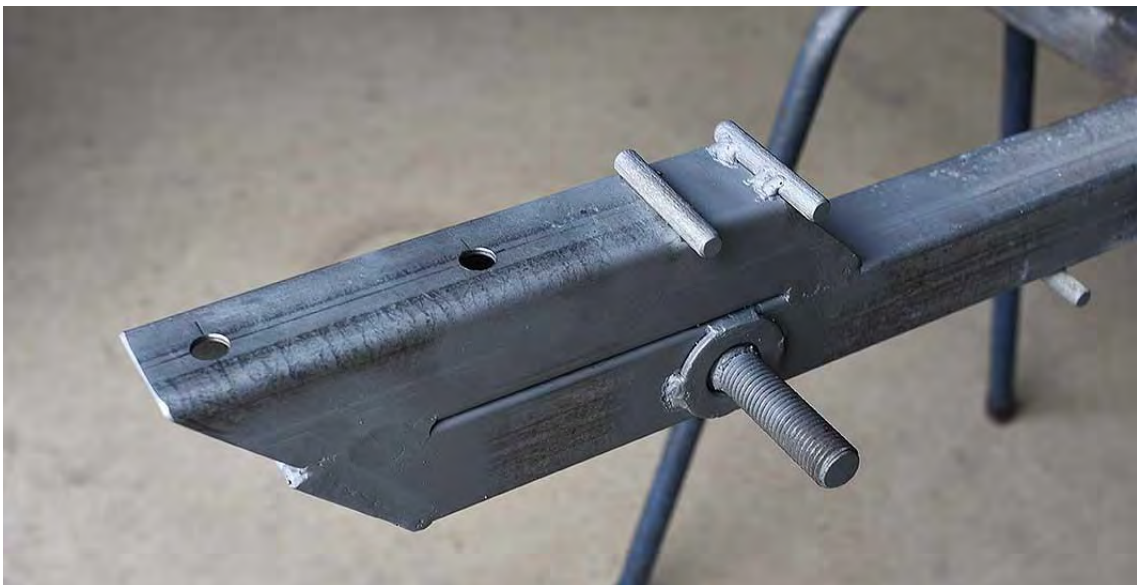
Picture 2: Front end of the drawbar with 20 mm threaded rod for the jockey stand and two 13mm holes for bolts to fix the trailer coupling.
